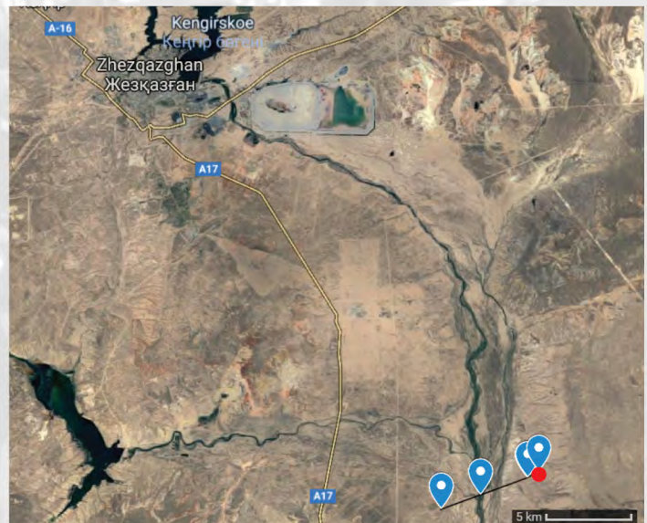
The landing trajectory of the SOYUZ MS-10 landing module based on the position data provided by the 406 MHz beacons. The landing position of the landing module is marked with a red dot.
